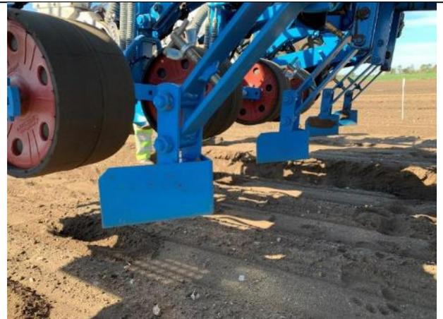
Front plough lowered so that it presses into loose soil and pushes it to the sides before the front wheel.
